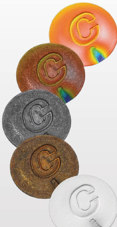
Five smart visualization modes (false color, stack, stack & false color, true color or directional luminance) are always within reach in the main screen.
