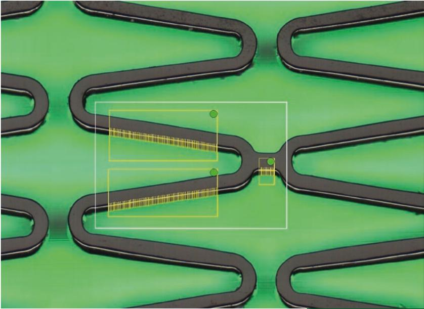
Images are processed to detect the light transitions that define the device limits (points A & C), the transition from outer to lateral surface (point B), and the reflection halo generated in the rounded edge of the device. The wall thickness and edge radius are accurately determined by the relative positions between these points.
